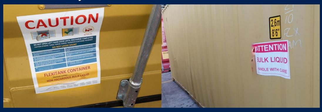
Marking of the container with appropriate labelling in the door area (work safety) as well as on the roof, as an indication for the van carrier/crane operator.
