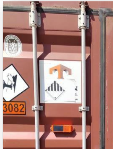
MP Mark sideways, Class 9 Placard too small
