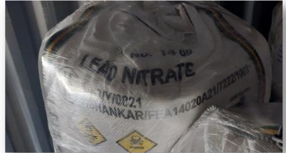
Missing Marine Pollutant (MP) Marks, Toxic Label is yellow (should be white)
